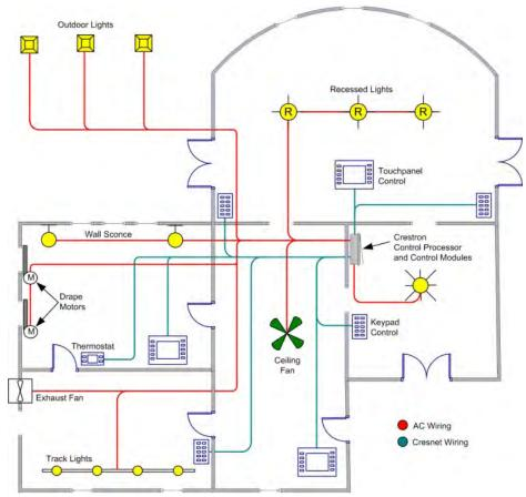
A Centralized Wiring System
